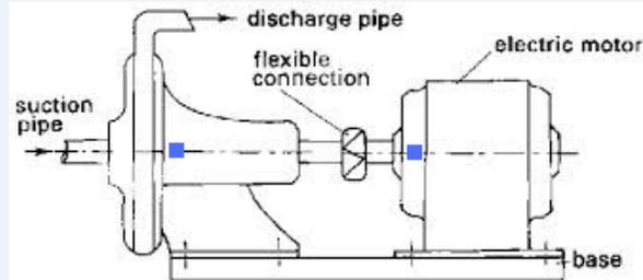
**Figure 2., Typical Mounting Locations for VTB-Sensor, 3-Axis Digital Transmitter on a Motor/Pump Set**
